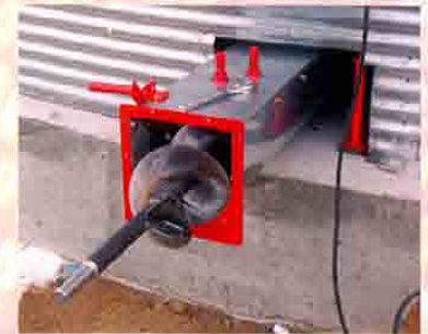
1/4-Inch (6-mm) Thick Auger Flight Is Easily Removed And Reinstalled From Outside The Bin
