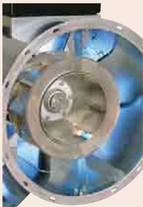
Dynamically balanced aluminum centrifugal wheel features advanced air foil blade design to efficiently handle low airflows at medium to high static pressures.
