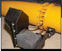
**Rugged Drive System** with positive sprocket rail drive for no-slip operation and more pushing torque.
