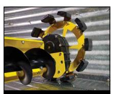
Highly Refined Drive Wheel Patent pending open-style design. 16:1 reduction ratio maximizes longevity.
