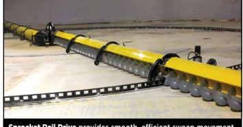
**Sprocket Rail Drive** provides smooth, efficient sweep movement. Dual arm option provides *MAVERIK*® *HTF Single Pass. Swept Twice.*<sup>™</sup> clean-up.
