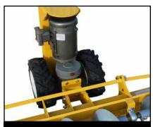
Weighted Tractor Drive offers greater traction and has more power to help drive the sweep into the grain. Weight on the drive is adjustable.
