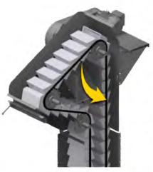
EZ-Flow™ Bucket Elevators move product with buckets fastened to two lengths of chain. The elevator's chain runs significantly slower than a traditional belt system allowing it to use free-gravity discharge. As the bucket and chain runs over the head sprocket, material gently pours out of the bucket into a discharge on the side of the elevator head.
