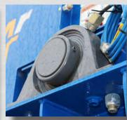
**Head Bearings** Heavy-duty pillow block bearings are externally mounted on all models.
