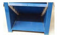
EASY CLEAN-OUT BOOT All EZ-Flow™ models feature Clean-Out Doors that slide open for easy access to the boot floor for cleaning.
